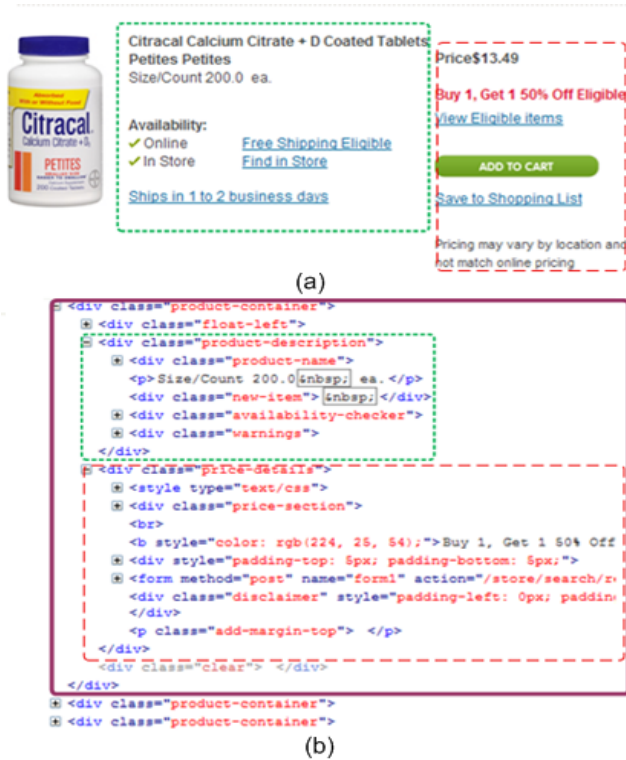
Figure 3. (a) A Search Result Item. (b) DOM tree node (highlighted using solid rectangle) for the search result item. Childnodes of this search result item with similar structure are highlighted using green and red dotted rectangle. This DOM tree node is a pattern node since its child nodes have similar tag distributions. Each of the search result items in Figure 2 are identified as pattern node, and their common ancestor becomes search result node containing search result items.
